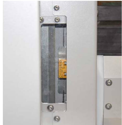
Integrated safety limit switch
