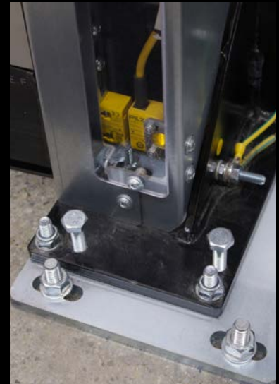
Integrated safety limit switch
